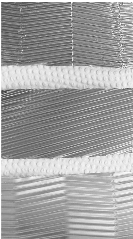
Fig. 3. Corrugation patterns employed in the manufacture of catalyst support structures: 150 cpsi Herringbone TI (top), 100 cpsi Skew pattern (middle) and TI 160 cpsi Herringbone APT SK (bottom).
